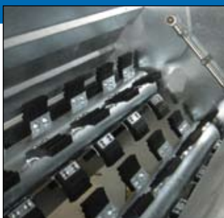
Enthaarungswalzen / Dehairing rolls
