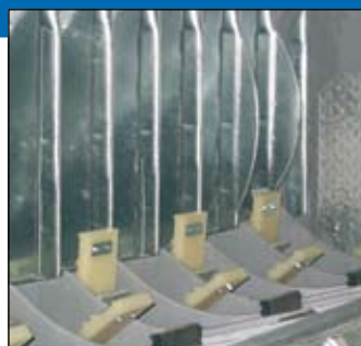
Enthaarungswalzen / Dehairing rolls
