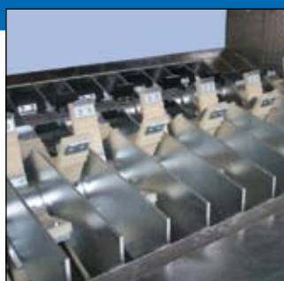
Enthaarungswalzen / Dehairing rolls
